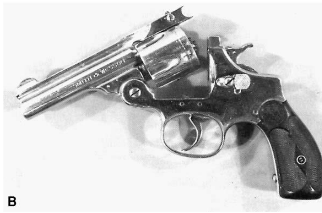
A) A 9-mm revolver, swing-out type, with cylinder swung open exposing chambers; (B) break-top revolver with action open.
